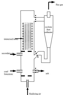
Figure 1. The scheme of the CFB combustor.
