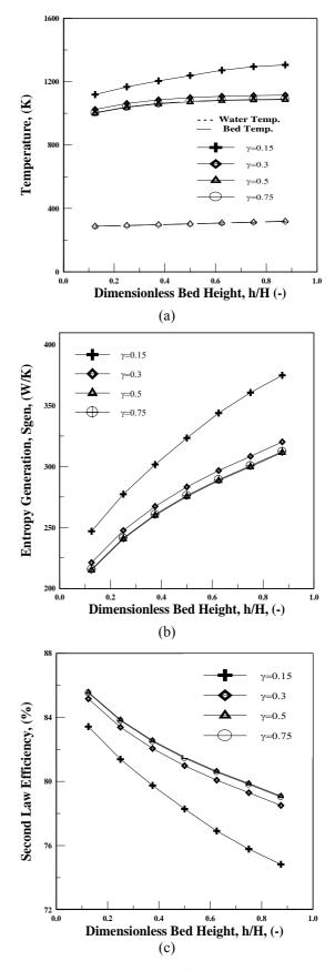
Figure 5. Variation of bed temperature (a), entropy generation (b), and second law efficiency (c) along the bed height.
