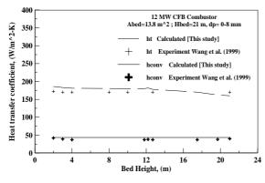
*Figure 4. Variation of heat transfer coefficients in the combustor.*
