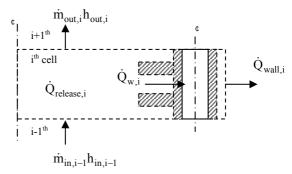
Figure 2. The energy balance of the control volume for immersed surfaces.
