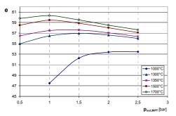
Figure 4. Exergetic efficiency as function of  $p_{out,MPT}$  (Cycle n°3).
