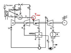
*Figure 3. Plant layout of the ZECOTECH<sup>®</sup> cycle.*
