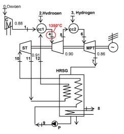
Figure 1. Plant layout of Cycle n°1.
