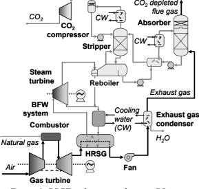
Figure 6. CCGT with post-combustion  $CO_2$ capture.
