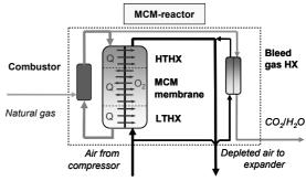
*Figure 2. MCM-reactor build-up.*
