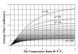
Figure 7. The entropy coefficient n versus the temperature ratio  $\theta$  for BR ( $T_S$ ) incident on a GR surface ( $\varepsilon$ , T);  $\theta > 1$
