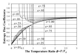
Figure 10. The entropy coefficient n versus the temperature ratio  $\theta$  for GR ( $\varepsilon$ ,  $T_s$ ) incident on a blackbody surface (T)
