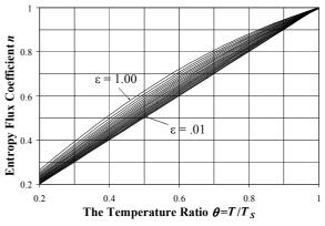
Figure 8. The entropy coefficient n versus the temperature ratio  $\theta$  for BR ( $T_s$ ) incident on a GR surface ( $\varepsilon$ , T);  $\theta < 1$
