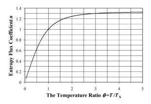
Figure 3. The entropy coefficient n versus the temperature ratio  $\theta$  for BR (T<sub>s</sub>) incident on a BR surface (T)
