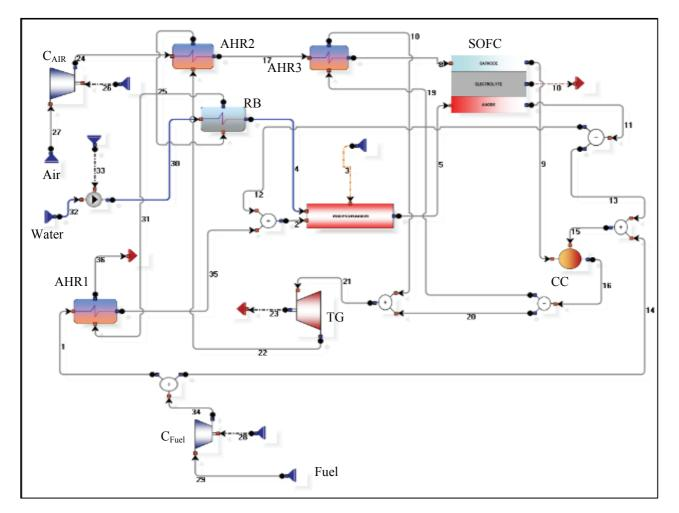
Figure 2. CAMEL- Pro<sup>™</sup> Flow Sheet of the SOFC/GT Hybrid System.
