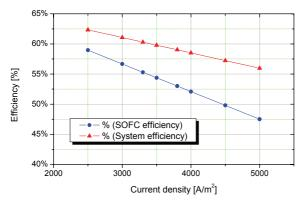
Figure 4. System Performance with Variable Fuel Cell Load.
