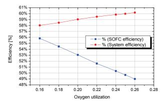
*Figure 5. System Performance with Variable Oxygen Utilization.*
