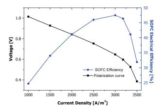
Figure 1. Polarization Curve and SOFC Efficiency.
