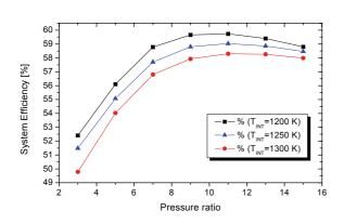
*Figure 3. System Performance with Variable SOFC Pressure and Turbine Inlet Temperature.*
