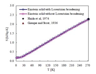
Figure 5. Entropy of ice. The curves with open circles and open squares are from the modified Einstein model with same frequency parameters as in Figure 3. Entropy data by Haida et al. (1974) and Giauque and Stout (1936) are obtained by graphical integration of ice heat capacities at 273.16 K and 273.10 K, respectively. The residual entropy at 0 K, 0.19 kJ/kg-K, is included in all the calculations.
