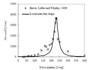
Figure 2. Absorption coefficient of ice Ih at 100 K.
