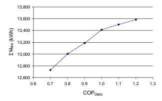
Figure 9. Effect of the nominal value of the absorption chiller COP on the total cooling energy supplied by the chiller.
