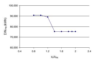
Figure 15. Effect of the cost of fuel on the total electric energy supplied by the cogeneration unit.
