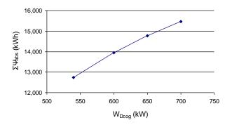
Figure 12. Effect of the nominal electric power of the cogeneration unit on the total cooling energy supplied by the chiller.
