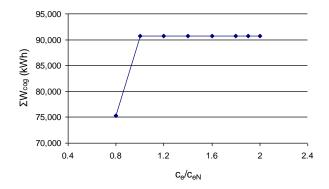
Figure 16. Effect of the cost of electricity on the total electric energy supplied by the cogeneration unit.
