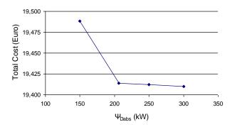
Figure 11. Effect of the nominal cooling power of the absorption chiller on the total cost for covering the energy needs.
