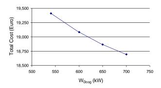
Figure 13. Effect of the nominal electric power of the cogeneration unit on the total cost for covering the energy needs.
