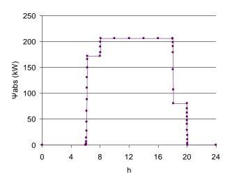
Figure 7. Change of the cooling power of the absorption chiller during a typical day in July.
