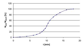
Figure 2. Gompertz function for load increase.
