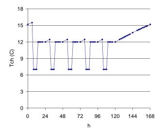
Figure 8. Change of the temperature in the cold water storage tank during a typical week in July.
