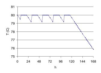
Figure 5. Change of the temperature in the hot water storage tank during a typical week in January.
