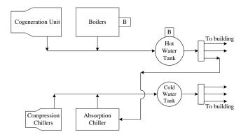
Figure 1. Simplified diagram of the energy system (only the supply lines of hot and cold water are depicted).
