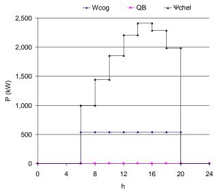
Figure 6. Change of the operating power of the cogeneration unit, the boilers and the compression chillers during a typical day in July.
