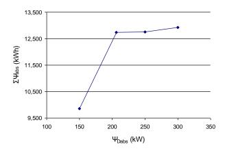
Figure 10 Effect of the nominal cooling power of the absorption chiller on the total cooling energy supplied by the chiller.
