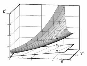
Figure 4. Depiction of the available energy of a body-and-medium (exergy of a body).
