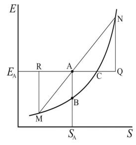
Figure 2. Depiction of  $E_{min}$  vs. S at fixed V, of available energy, and of available entropy
