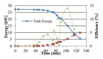
*Figure 8. The variation of the exergies and efficiencies in the separation operation.*
