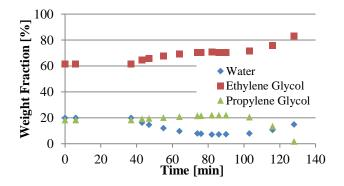
*Figure 7. The components present in the reboiler tank during the distillation process.*
