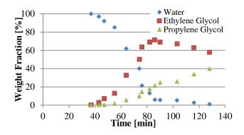
*Figure 6. The components present in the distillate during the distillation process.*
