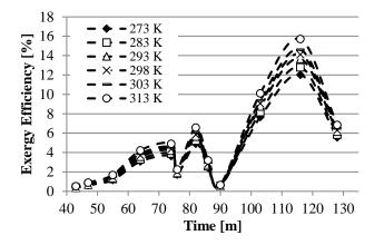
Figure 10. Parametric investigation of reference temperature on exergy efficiency.
