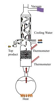
Figure 1. The scheme of the experimental setup.
