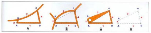
Figure 1. The simplest plane mechanism samples consisting of four bars [4]
