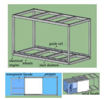
Figure 13. Cell sliding system construction drawings [22]
