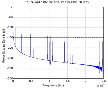
Figure 1. PSD diagram for a single excitation force which is set to first mode frequency
