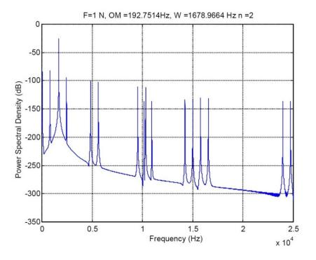
*Figure 2. PSD diagram for a single excitation force which is set to third mode frequency with zero phase difference*
