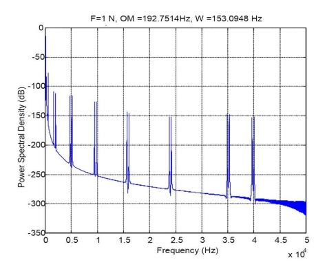
*Figure 4.* PSD diagram for two different excitation forces which have  $\pi/6$  phase difference
