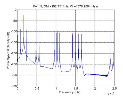
*Figure 3.* PSD diagram for a single excitation force which is set to third mode frequency and phase difference is  $\pi/2$
