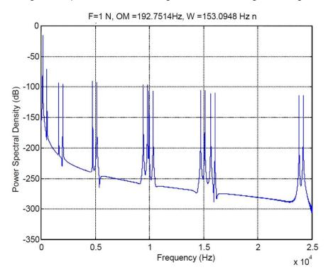
*Figure 5. PSD diagram for two excitation forces which have different excitation locations and different phase differences*
