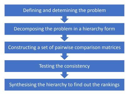
Figure 1: Flowchart of the AHP application steps
