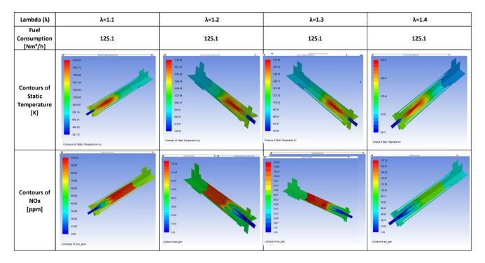
Figure 7. Contour plots of Static Temperature and NOx mole fraction distributions with varying excess air ratio.
