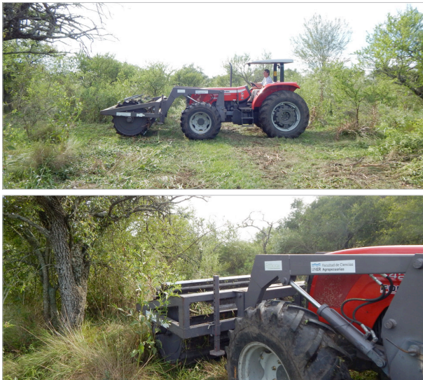
Figure 3. Roller-chopping designed by the Chair Ecology of Agricultural Systems (FCA-UNER)
