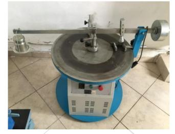
Figure 1. Bohme abrasion test device
