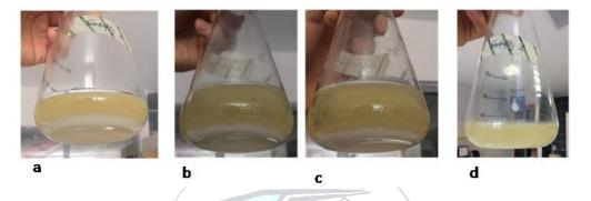
Figure 3. CaCO<sub>3</sub> formation during incubation (after; a)1 hour; b) 2 hours; c) 1 day; d) 1 week)
