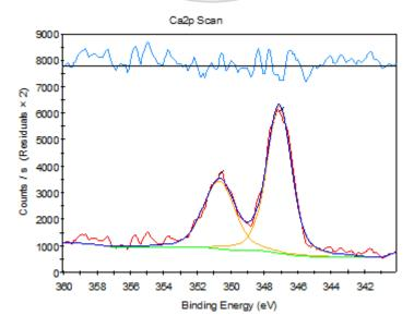
Figure 7. XPS spectrum of Ca in solidified sand
