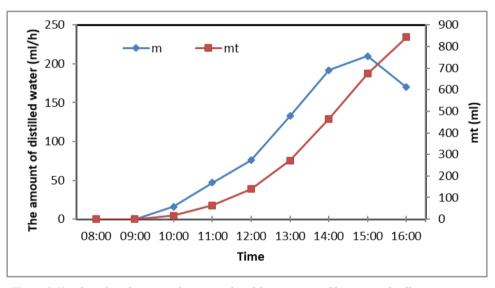
Figure 9. Hourly and total amount of water produced for conventional basin-type distiller
