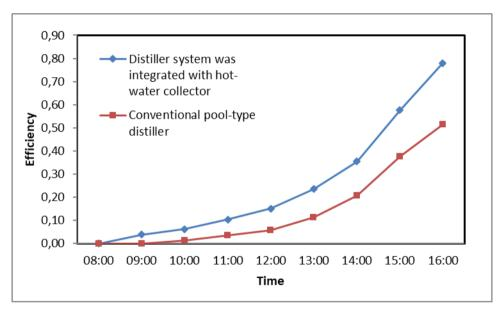
Figure 14. Efficiencies of solar supported integrated water heating-distillation system and conventional basin type
