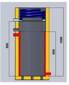
Figure 4. Dimensions of tank-type distiller (mm)
