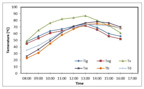
Figure 8. Change of temperatures in solar supported integrated water heating-distillation system with time
