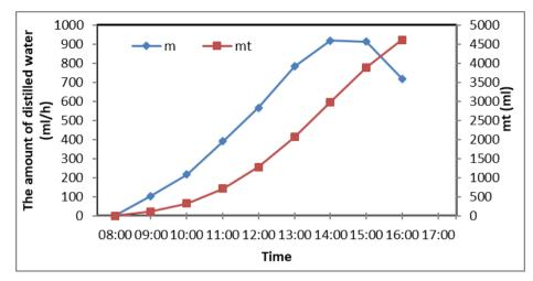
Figure 10. Amount of hourly and total produced distilled water in solar supported integrated water heating-distillation system
