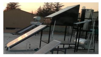
Figure 2. Photo of distiller system integrated with hot water collector
