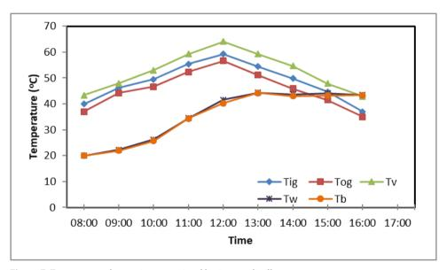
Figure 7. Temperature changes in conventional basin-type distiller
