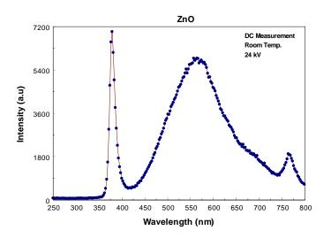
Figure 2. The CL spectrum of pure ZnO at room temperature.
