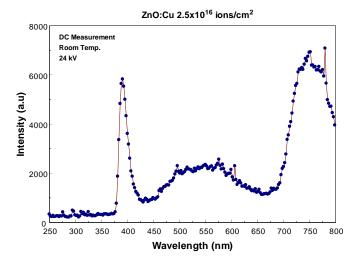
**Figure 3.** CL spectrum of Cu implanted ZnO with concentration 2.5x10<sup>16</sup> ions/cm<sup>2</sup> when bombarded with 24 kV electron beam.
