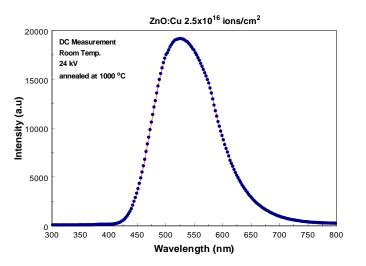
Figure 4. CL spectra of ZnO with 2.5x10<sup>16</sup> ions/cm<sup>2</sup> Cu ions implanted and annealed in air.
