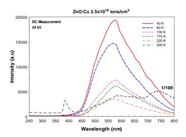
**Figure 5.** The DC CL spectra of the Cu implanted ZnO at  $2.5 \times 10^{16}$  ions/cm<sup>2</sup> dose crystal at different temperatures.
