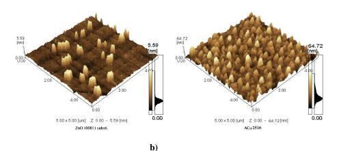
**Figure 1. a)** The AFM photo of single ZnO (0001) crystal **b**) The AFM photo of ZnO: Cu  $2.5 \times 10^{16}$  ions/cm<sup>2</sup> sample after 1 hour annealing process.
