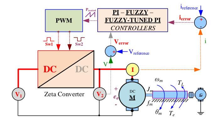
Figure 1. Starting Current PI, Fuzzy and Fuzzy-Tuned PI controllers and Zeta Converter Controlled Serial Connected DC Motor System Block Diagram
