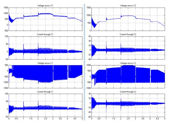
Figure 11. Current and voltage changes of L<sub>1</sub>, L<sub>2</sub>, C<sub>1</sub> and C<sub>2</sub> elements in the zeta converter circuit.
