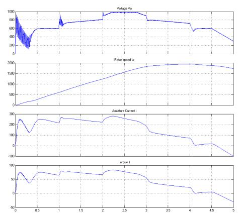
**Figure 16.** Variation of the output voltage v<sub>o</sub>, w motor speed, i<sub>A</sub> motor current and T<sub>e</sub> torque value of the motor with time controlled by Fuzzy Logic controlled Zeta Converter.
