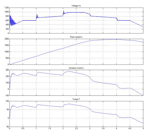
Figure 13. Variation of the output voltage vo, w motor speed, i<sub>A</sub> motor current and T<sub>e</sub> torque value of the motor with time controlled by Fuzzy Logic controlled Zeta Converter.
