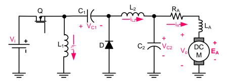
Figure 3. Zeta Converter-fed Serial DC motor load.
