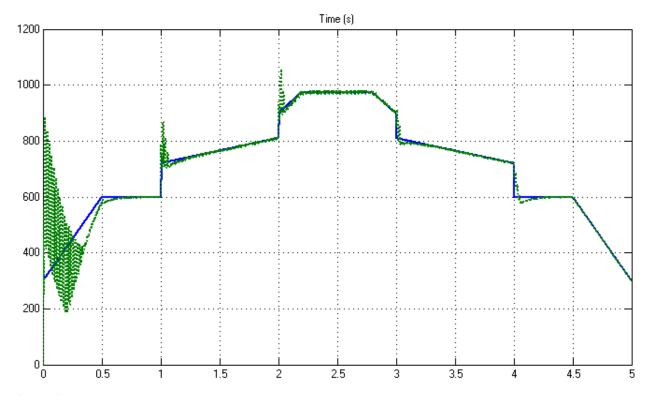
Figure 9. Variation of the output voltage  $v_o$  over time with the reference signal of the Zeta converter with PI
