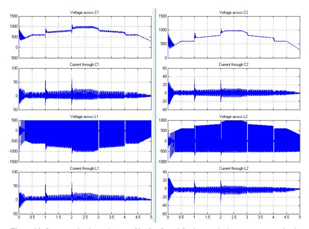
Figure 14. Current and voltage changes of L<sub>1</sub>, L<sub>2</sub>, C<sub>1</sub> and C<sub>2</sub> elements in the zeta converter circuit.
