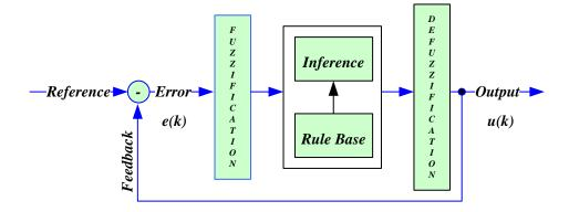
Figure 5. Basic configuration of a FLC.
