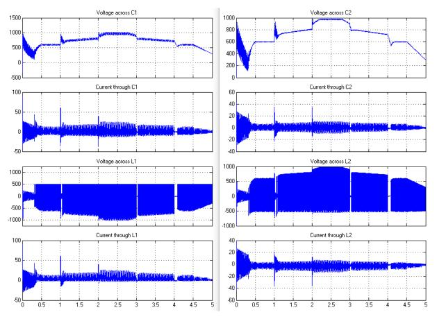
Figure 17. Current and voltage changes of L<sub>1</sub>, L<sub>2</sub>, C<sub>1</sub> and C<sub>2</sub> elements in the zeta converter circuit.
