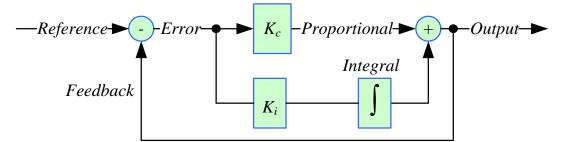
Figure 4. PI Controller Block Diagram
