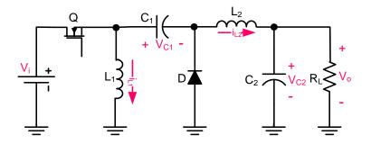
Figure 2. Circuit diagram of PWM Zeta Converter.
