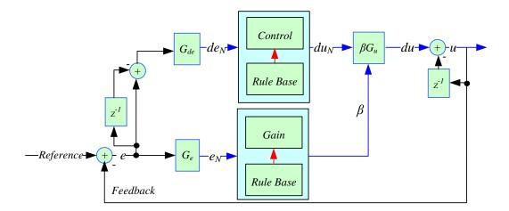
Figure 6. Basic configuration of a FT-PIC.
