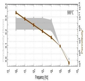
Figure 5 APA graphs of the temperature-dependent change in conductivity and Permittivity -received %66Ni Plated  $Si_3N_4$  Composite at 800°C sintered.
