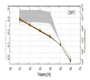
Figure 6 APA graphs of the temperature-dependent change in conductivity and Permittivity -received %66Ni Plated Si<sub>3</sub>N<sub>4</sub> Composite at 1200°C sintered
