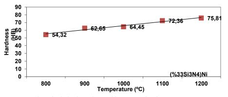
Figure 2. The hardness change with respect to sintering temperature
