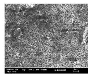
Figure 7 SEM micrographs of as-received Ni Plated  $\rm Si_3N_4.~Mag.2kX~800^{\circ}C$
