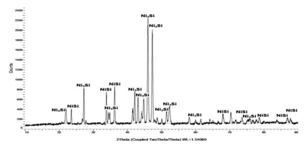
Figure 10 X-ray diffraction patterns of the (Si<sub>3</sub>N<sub>4</sub>)%66Ni sintered at 1200°C
