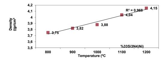
Figure 1. The density change with respect to sintering temperature
