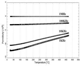
Figure 4 APA graphs of the temperature-dependent change in permittivity -received %66Ni Plated  $Si_3N_4$  Composite at 1200°C sintered.
