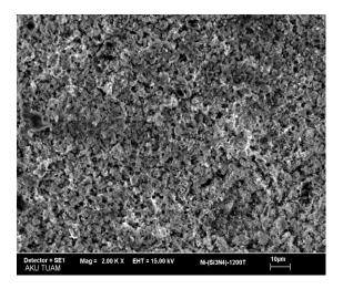
Figure 8 SEM micrographs of as-received Ni plated  $Si_3N_4$ . Mag.2kX 1200°C
