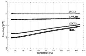
Figure 3 APA graphs of the temperature-dependent change in permittivity -received %66Ni Plated  $Si_3N_4$  Composite at 800°C sintered.
