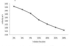
Fig.4 Outlet velocity of abrasive with different volume fraction
