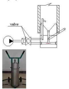
Fig.5 Assembly drawing of abrasive mixing chamber
