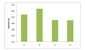
Fig.2 The max velocity of four abrasive mixing chambers
