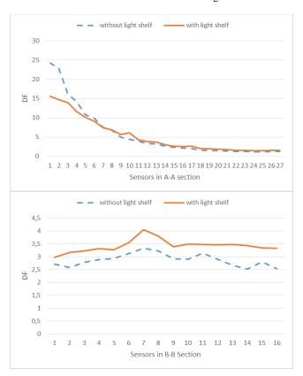
Figure 7. DF value distributions in A-A and B-B sections for with and without light shelf conditions.
