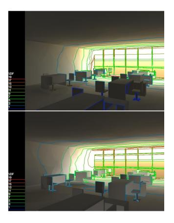
Figure 8. Volumetric distribution of DF with (right) and without (left) light shelf.
