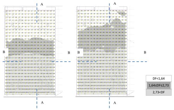
Figure 6. Distribution of daylight interiors with & without light shelf.
