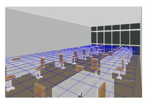
Figure 1. Sample Office, sensor placement on 75 cm height and light shelf on facade.
