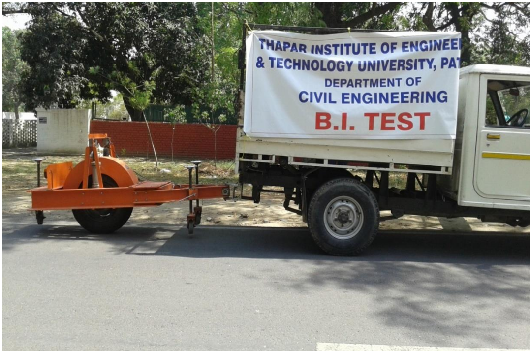
Fig. 1. Bump integrator test (Roughness test)
