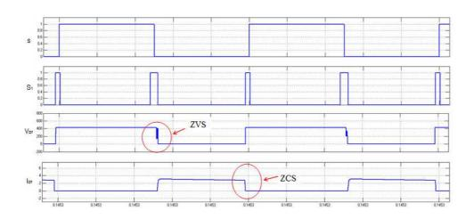
Figure 16. Switching signal of the main switch (S), switching signal of the auxiliary switch ( $S_1$ ), the main diode voltage ( $V_{DF}$ ), the main diode current ( $I_{DF}$ )
