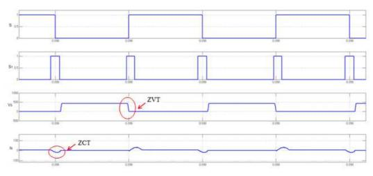
Figure 11. Switching signal of the main switch (S), switching signal of the auxiliary switch ( $S_1$ ), the main switch voltage ( $V_S$ ) the main switch current ( $I_S$ )
