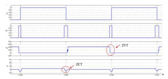
Figure 14. Switching signal of the main switch (S), switching signal of the auxiliary switch ( $S_1$ ), the main switch voltage ( $V_S$ ) the main switch current ( $I_S$ )
