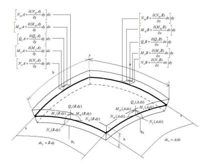
Figure 2. Forces and moments on shell element
