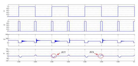
Figure 12. Switching signal of the main switch (S), switching signal of the auxiliary switch ( $S_1$ ), the auxiliary switch voltage ( $V_{S1}$ ) the auxiliary switch current ( $I_S$ )
