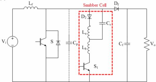
Figure 8. The ZVZCT DC-DC converter [8]
