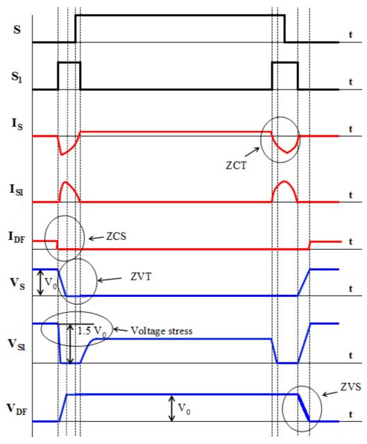
Figure 9. Waveforms of the semi-conductors in the converter [8]
