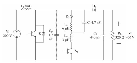
Figure 13. The model of ZVZCT Converter-II used in simulation [8]
