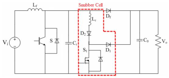
Figure 4. The basic ZVT converter circuit [5]
