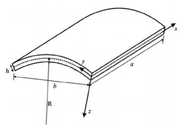
Figure 3. A cylindrical shell element
