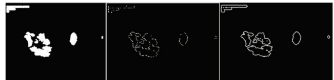
Figure 3. (a) Image after thresholding, (b) image after Sobel algorithm, and (c) image after dilation
