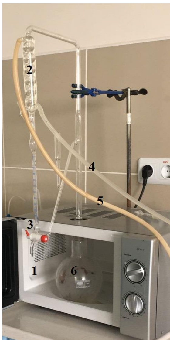
Figure 1. Microwave-assisted cleverger setup (1-Microwave oven, 2-Cleverger unit, 3-Tap, 4-Cooling water inlet, 5-Cooling water outlet, 6-Sample flask)
