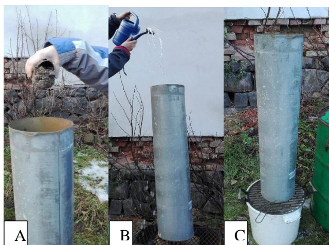
Figure 1. Research of infiltration of produced substrate containing cardboard and soil. A: Filling the tube by the substrate B: Rain simulation, C: Container for measuring outgoing water.
