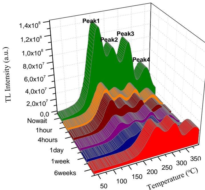
Figure 4. The TL glow curve for dental glass ceramic with respect to the fading.
