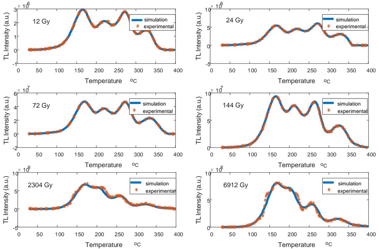
Figure 3. The TL glow curve of simulation and experimental results of glass ceramic as a function of dose response irradiated with  $\beta$ -source for 12, 24, 72, 144, 2304 and 6912 Gy at room temperature
