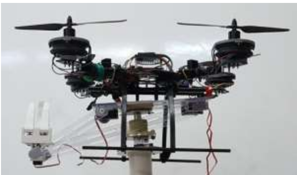
Figure 17. Manufactured mechanism, gripper and the electronic system installed on a UAV.
