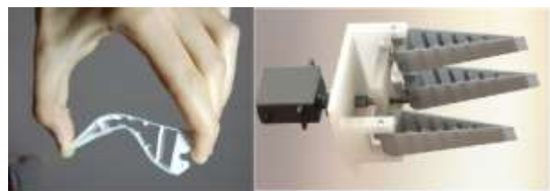
Figure 6. a) Flexible finger, b) Manufactured gripper with three fingers.
