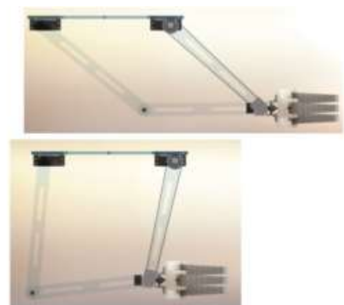
Figure 4. Mechanism at the position of grasping (up). Mechanism is at the position of balance (bottom).
