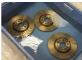
Figure 14. Rotors after crack test with thermal shock.
