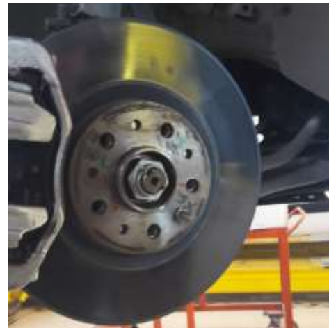
Figure 10. Assembled brake disc on vehicle after thermal shocked crack test on vehicle.
