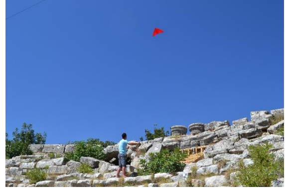
Fig. 16. Operation of taking aerial photos with kite
