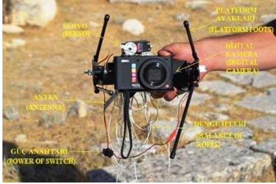
Fig. 13. Digital Camera and its carrying platform
