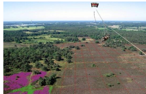
Fig. 9. Kite Aerial photography can be used to obtain more analyses and data. It is a low cost and effective method that is suitable for working in small regions (URL-23).
