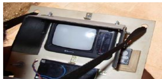
Fig. 12. Ground control unit with monitor (Altan, 2004)
