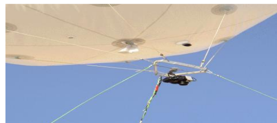
Fig. 11. Camera platform, camera, and balancing ropes under balloon (Altan, 2004)
