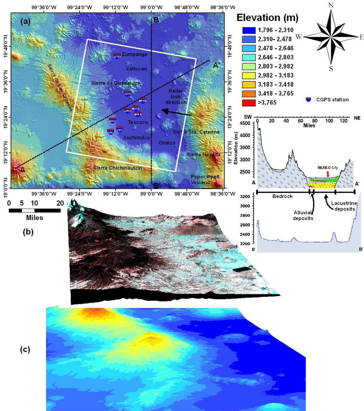
**Figure 1.** a) Mexico City topography map and installed CGPS stations in the metropolitan area. White rectangle shows the InSAR data coverage area in descending mode. b) 3D view of the study area with Landsat ETM+ imagery from 25/11/2005. c) 3D representation of Mexico City area (Poreh and Pirasteh, 2019)
