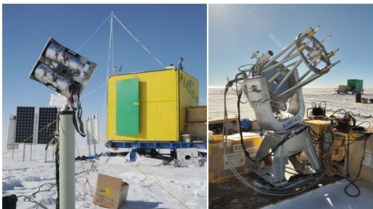
Figure 10. A year-round observation system for extrasolar planets (left) started operation, and seasonal observation with a 40-cm telescope (right) was carried out at Dome Fuji Station in the 2010–2011 austral summer season.
