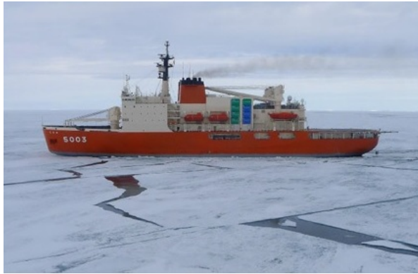
Figure 11. Japanese icebreaker Shirase, 134 meter in length and 12,500 tonne in displacement (photographed 16 February, 2013).
