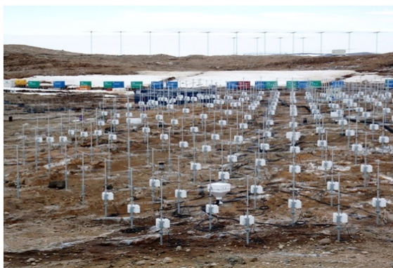
Figure 7. The PANSY radar system, including 1054 Yagi antenna elements, installed at Syowa Station in the 2010–2011 Antarctic season.
