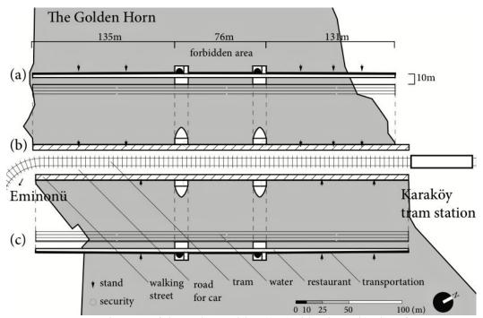
**Figure 3.** Diagram of the Galata Bridge; (a,c) side view, (b) view from top.
