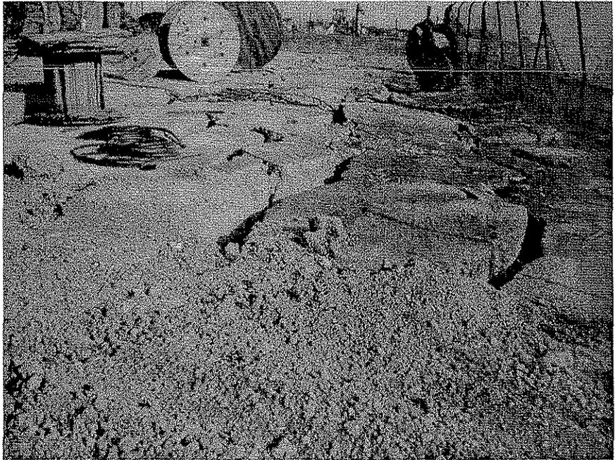
Figure 4. Pictures show the ruptures at (a) Kavaklı and (b) Tüpraş.
