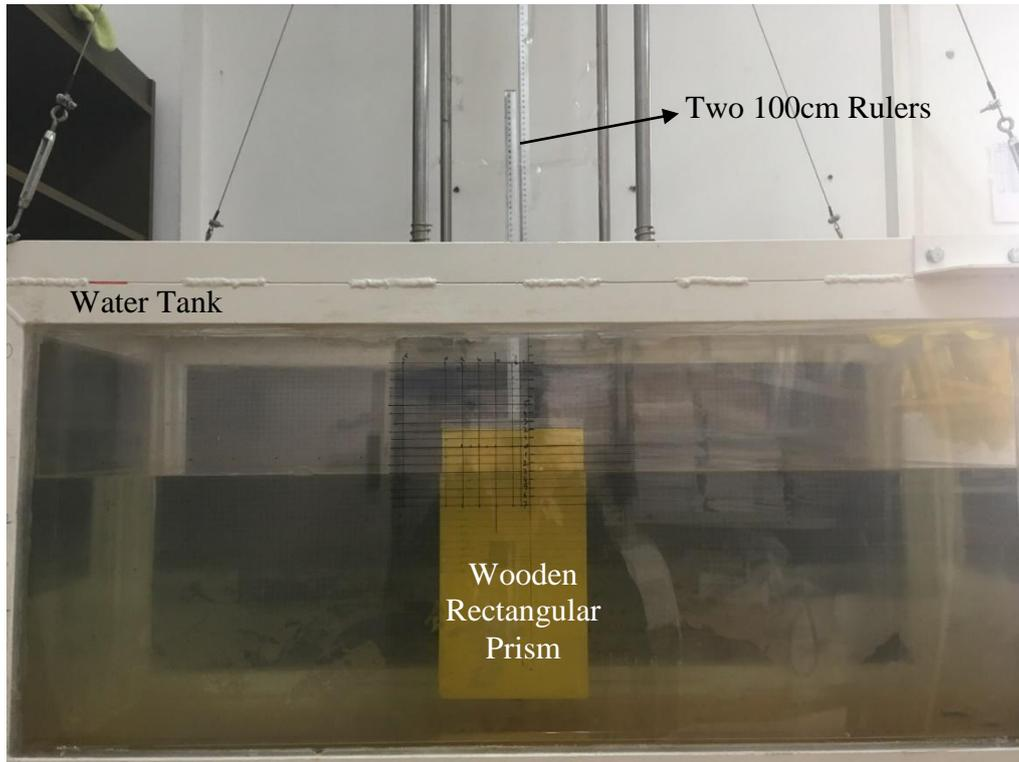
**Figure 5:** Snapshot of Second Section of the Experiment Setup
