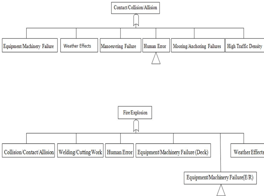
Fig. 5. FTA of contact/collision/allision category and fire/explosion category
