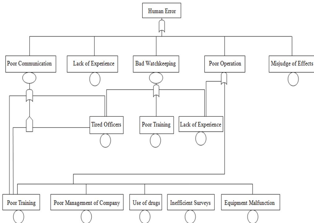
**Fig. 6.** FTA of human error for collision/contact/allision category
