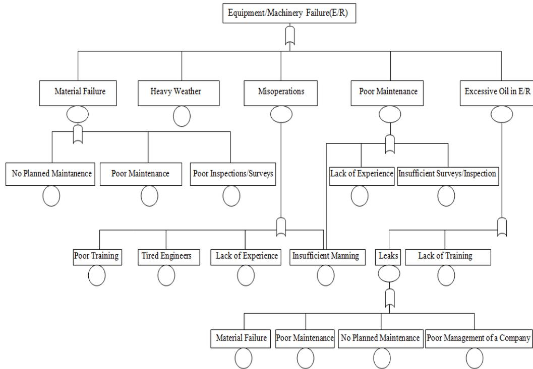
**Fig. 7.** FTA of equipment/machinery failure in engine room for fire/explosion category.
