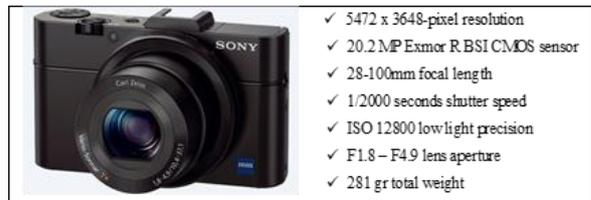
**Figure 3.** Technical specifications of the Sony RX100II compact camera.
