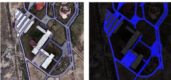
Figure 7. Roads detected on orthophoto
