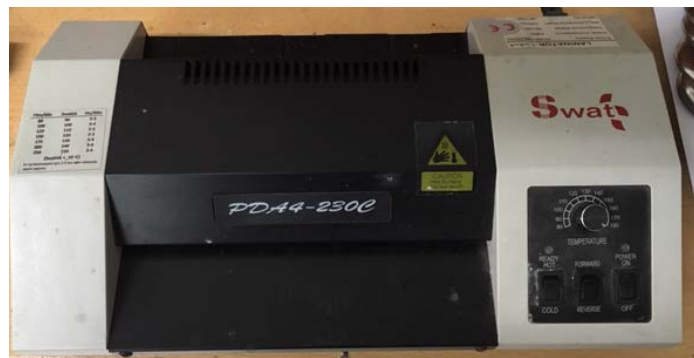
Figure 5. Laminating device used for the printed circuit.
