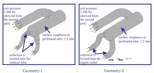
Figure-3: Modified Dry-Type Silencer Models
