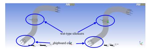
(a) Single İnlet (perp. and 45° inclined ) (b) Double İnlet (perp. and 45° inclined )
