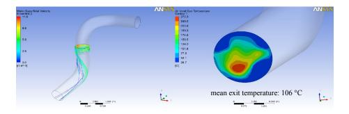
(a) Sea Water Streamlines (b) Temperature Contours at Shipboard Exit
