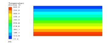
Figure-8: Temperature Distribution of Sheet Metal and Insulation Material
