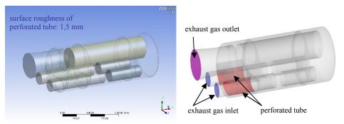
Figure-1: First Dry-Type Silencer Model
