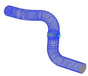
Figure-10: Wet-Type Silencer Model Mesh
