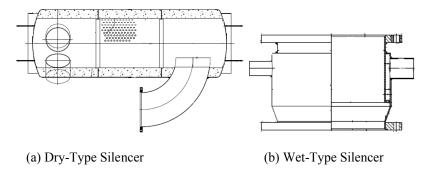
Figure-15: Technical Drawings Belonging to Dry and Wet-Type Silencers [6]
