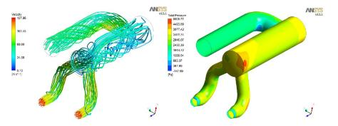
Figure-6: Stream Lines and Pressure Loss (Geometry-2)
