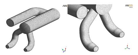
Figure-4: Modified Dry-Type Silencer Model Mesh (Geometry-2)
