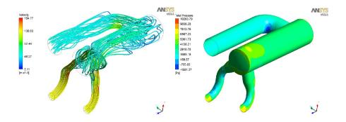
Figure-5: Stream Lines and Pressure Loss (Geometry-1)
