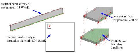
Figure-7: The Conditions in Thermal Analysis
