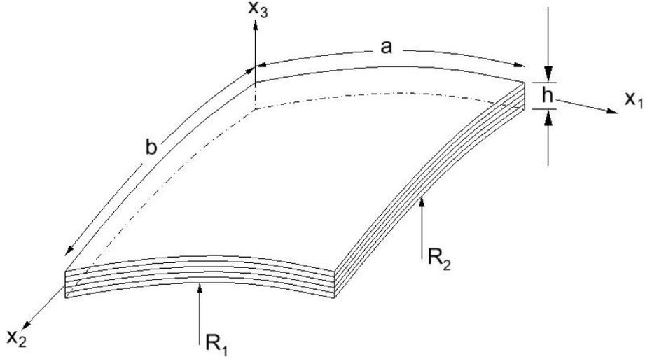
Figure 1. Geometry of a laminated plate.
