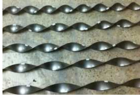
Figure 4. The twisted tapes inserts with tefflon rings
