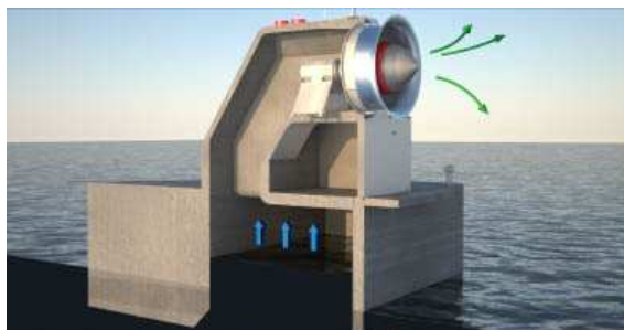
c. System schematic for two way turbine function Figure 3: Oscillating water column system
