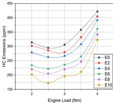
Figure 7. Variation of HC emission with engine load
