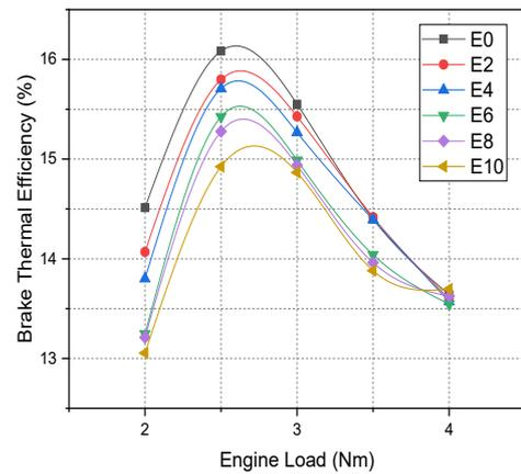
Figure 5. Variation of BTE with engine load
