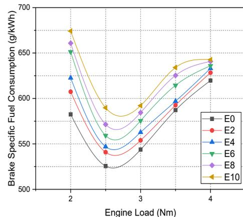
**Figure 3.** Variation of BSFC with engine load
