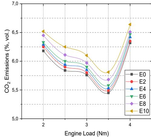
Figure 9. Variation of  $\text{CO}_2$  emission with engine load
