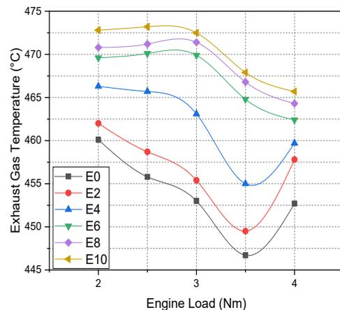
Figure 6. Variation of EGT with engine load
