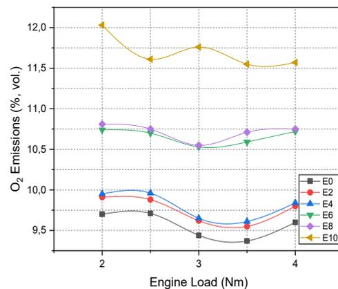
Figure 10. Variation of  $\text{O}_2$  emission with engine load
