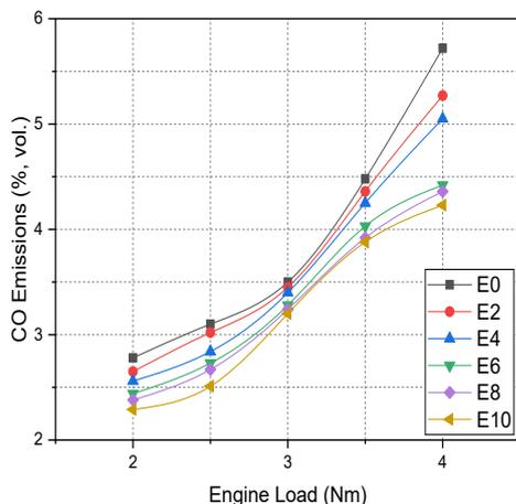
Figure 8. Variation of CO emission with engine load
