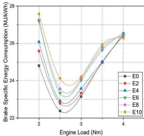
Figure 4. Variation of BSEC with engine load
