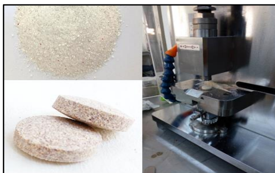
Figure 1: Direct compression of ferrous sulfate plus ascorbic acid effervescent tablets.
