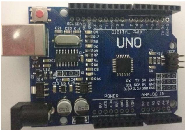
Figure 1 Arduino UNO microcontroller board
