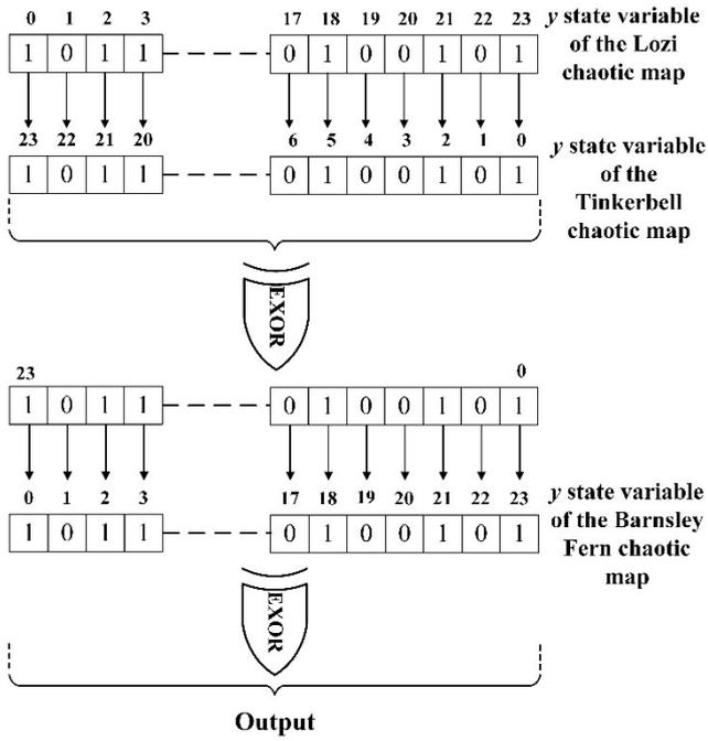
Figure 9 Second 24-bit algorithm of the RNG output
