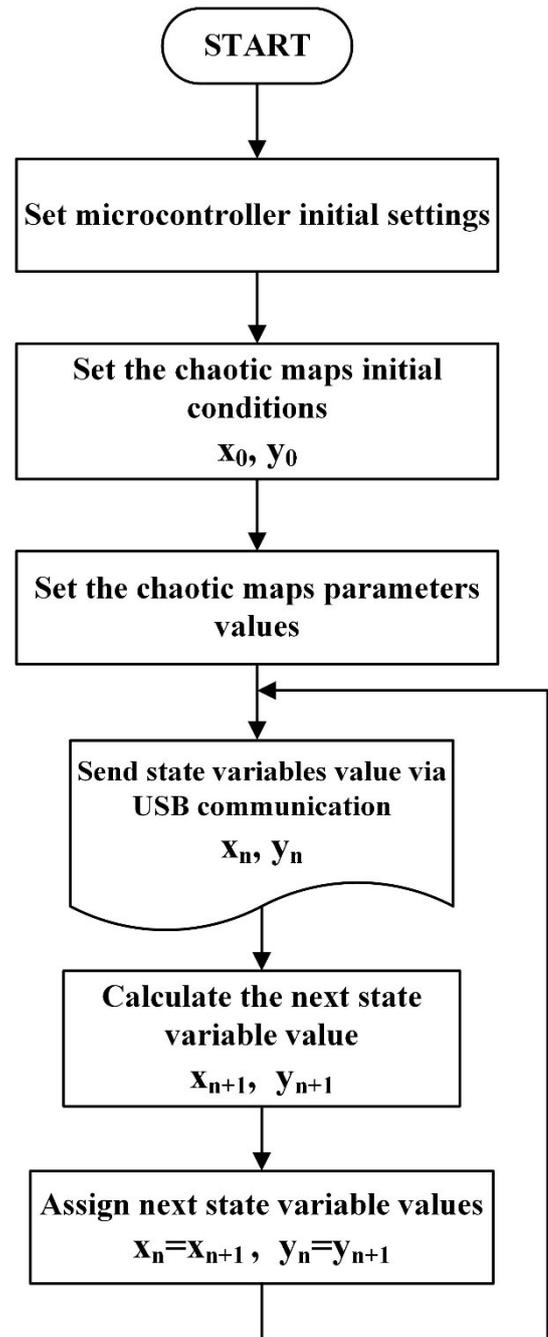
Figure 2 The flow chart of the microcontroller software
