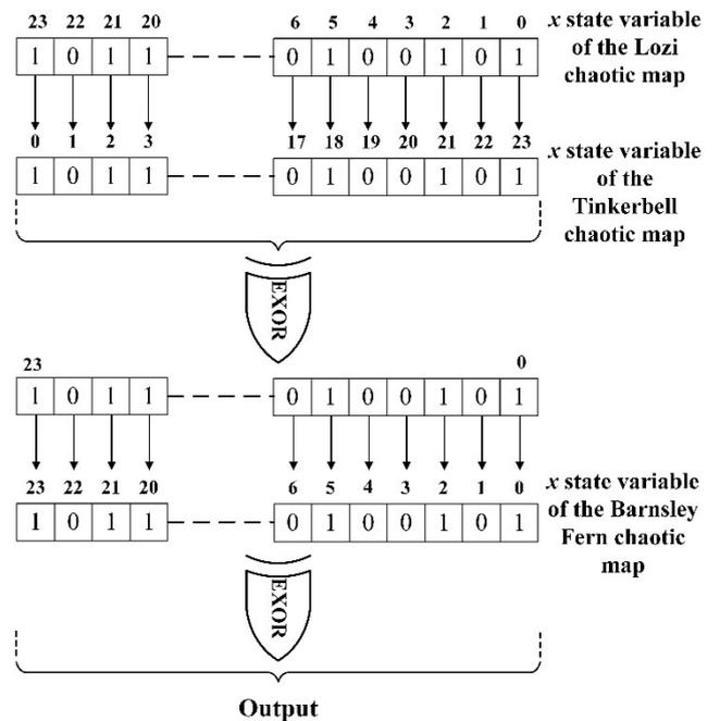
Figure 8 First 24-bit algorithm of the RNG output
