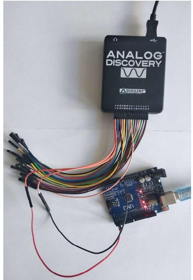
Figure 10 Measurement set-up of microcontroller based RNG output signal with a computer-based oscilloscope
