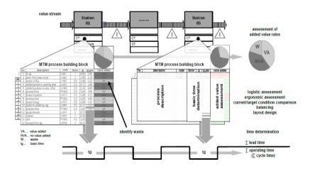
Figure 2. Principle of Value Stream Mapping and MTM Application (Kuhlang et al., 2008)
