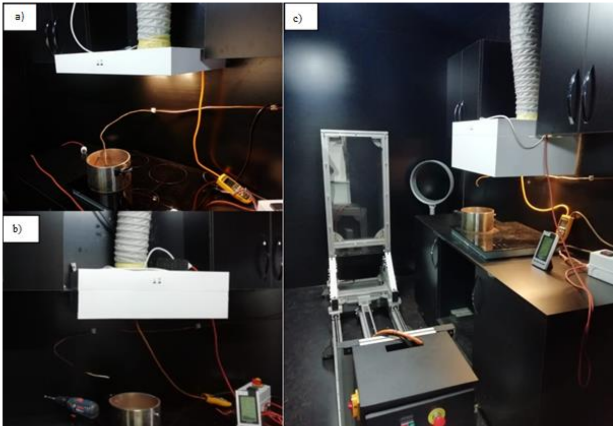
Figure 4. Odour extraction performance test. a) Without barrier, b) 10cm with Barrier, c) 20cm with Barrier.
