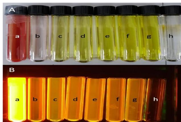
Figure 3 Image of CdSeTe QD/ BPB hybrid associates samples A) under sunlight, B) under florescent light. a-h shows the different ratio of hybrid associates QD: BPB , a) 100:0, b) 1:0, c) 1:0.25, d) 1: 0,5, e) 1: 1, f) 1:2, g) 1:3, h) 0:3.
